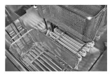
Thermostatically controlled tip-up heating elements, directly installed in the well.
